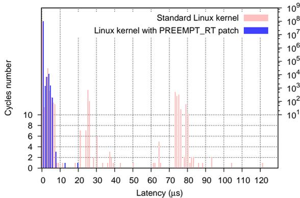
**FIGURE 4:** Histograms generated by NPT for  $10^8$  cycles on standard and PREEMPT\_RT patched kernels with LTTng-UST tracing
