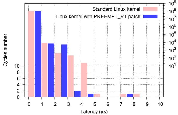
**FIGURE 8:** Histograms generated by NPT for  $10^8$  cycles on standard and PREEMPT\_RT patched kernels with modified LTTng-UST tracing
