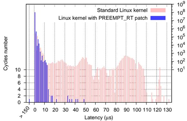
**FIGURE 5:** Histograms generated by NPT for  $10^8$  cycles on standard and PREEMPT\_RT patched kernels with LTTng kernel and UST tracings
