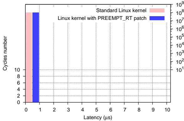
**FIGURE 3:** Histograms generated by NPT for  $10^8$  cycles on standard and PREEMPT\_RT patched kernels with LTTng kernel tracing
