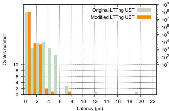
**FIGURE 7:** Histograms generated by NPT for  $10^8$  cycles on a PREEMPT\_RT patched kernel with original and modified LTTng-UST tracing
