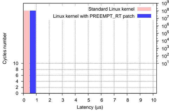
**FIGURE 2:** Histograms generated by NPT for  $10^8$  cycles on standard and PREEMPT\_RT patched kernels
