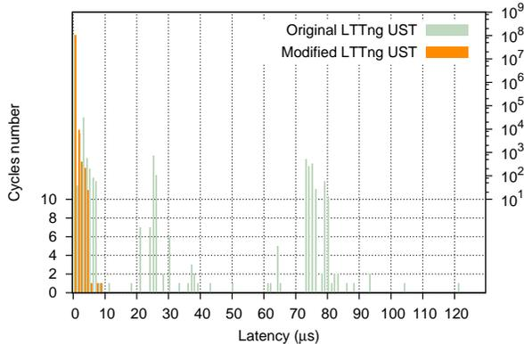
**FIGURE 6:** Histograms generated by NPT for  $10^8$  cycles on a standard kernel with original and modified LTTng-UST tracing
